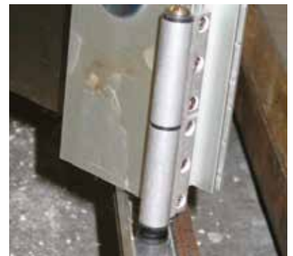
Picture 3: Sand and grit applied into bottom (33,000 cycles)
